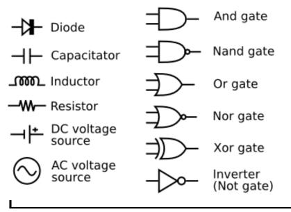
These symbols show some of the common circuit elements. A diode only lets current flow one way (the direction of the arrow). A resistor slows down the flow of current.
