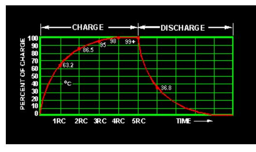
As this graph shows, the charging (or discharging) is essentially complete after 5 RC time periods.
